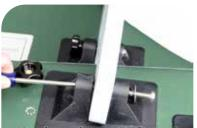
Knob and Bolt and Lock Washer Flat Washer this side this side
