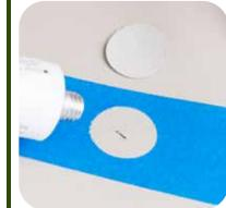
Apply glue to the patch and boat. Allow to dry 15 minutes. Glue must be dry to the touch. If glue layer is thin, apply second coat, allow to dry 15 minutes.
