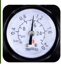
Pressure gauge will not register until chamber begins to get pressurized.
