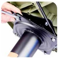
Attach pedestal to seat swivel with the short 1/2" screws and locking nuts. Hand tighten nuts until all screws have been inserted. Use 7/16" wrench or adjustable wrench to secure the pedestal.
