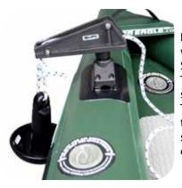
Line up the slot in the stem with the key in the base. Slide stem into base. To spin the anchor lock, lift slightly and turn it. To remove it, pull it up and turn it until the key and slot line up and pull it out of base.
