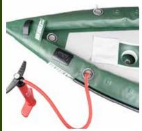
With valve stem in the up position, insert adapter, push down firmly and twist clockwise. Inflate floor chamber to full pressure. At this time, partially inflate the sides. Sides need to be soft so grommet holes can be lined up with transom holes.
