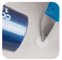
Apply patch to the boat. Smooth with finger or a smoothing tool such as a spoon, handle of a utility knife, or screwdriver. For best results, heat patch with a hair dryer 10-20 seconds and smooth with tool.
